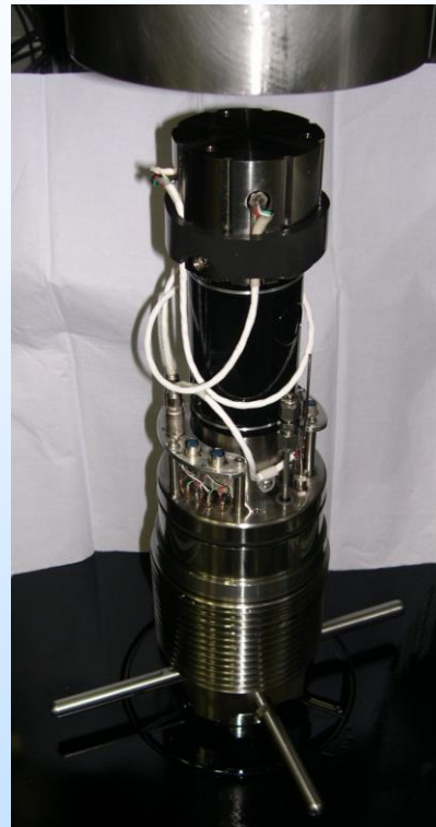
Dual Purpose Core Holder Assembly (for permeability and sonic velocity measurements)
