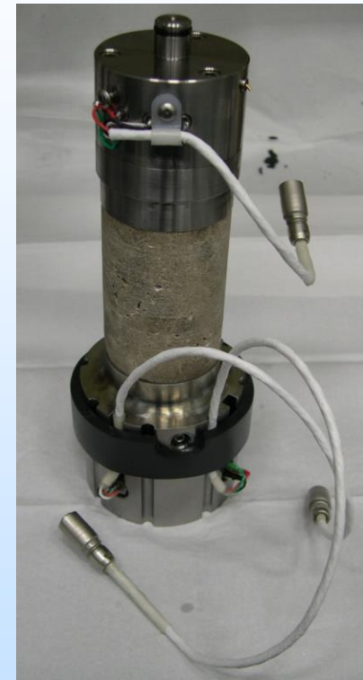
Dual Purpose Core Holder Assembly (for permeability and sonic velocity measurements)
