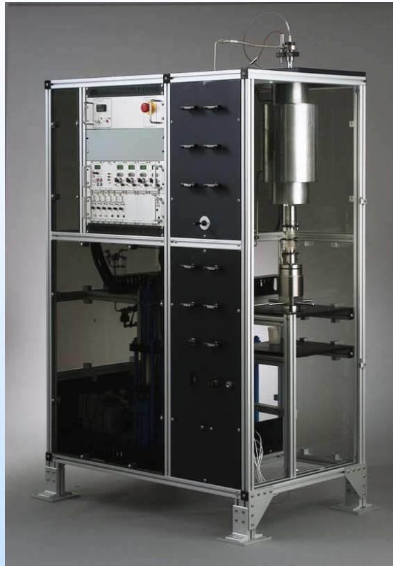
AutoLab 1500 automatic servo hydraulic triaxial system (NER, Inc) simulates in-situ conditions up to 90MPa overburden and 50MPa pore pressure
